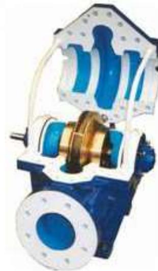
Gbr. 3.1.2.1.2. Pompa split casing in-line horizontal single stage
